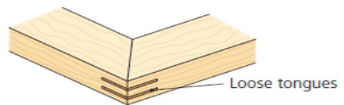
Mitre joint with loose tongues
